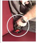
**Step 3**Click the SafeGuard MiniConnector into the LATCH bar
