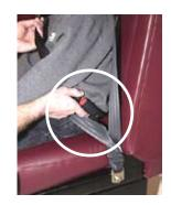
**Step 5**Click the other SafeGuard Mini-Connector into the LATCH bar on the opposite side of the seat.
